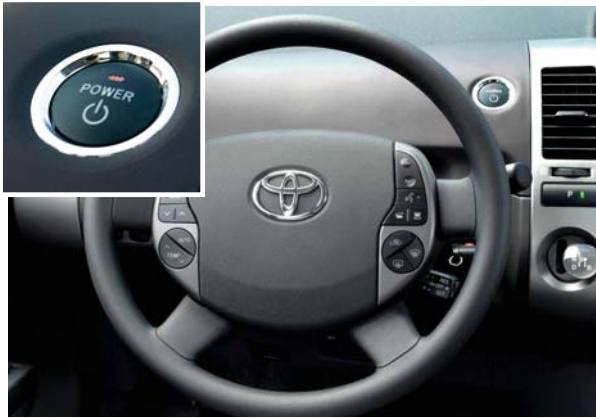
The dashboard on the Prius features something not seen on ordinary cars—a power button, inset.
